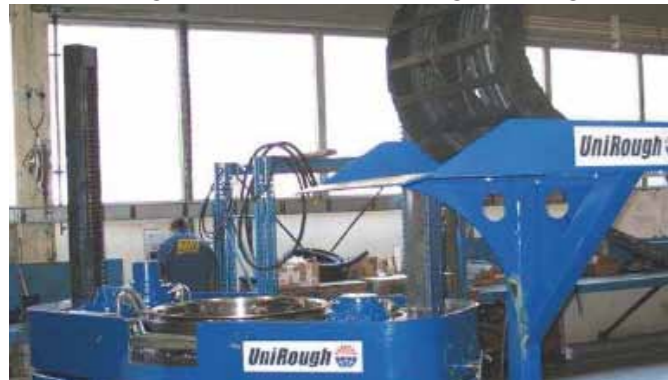
igus® e.chain® series 600 and igus® drylin® linear slides on a roughneck "V-Tech UniRough"
