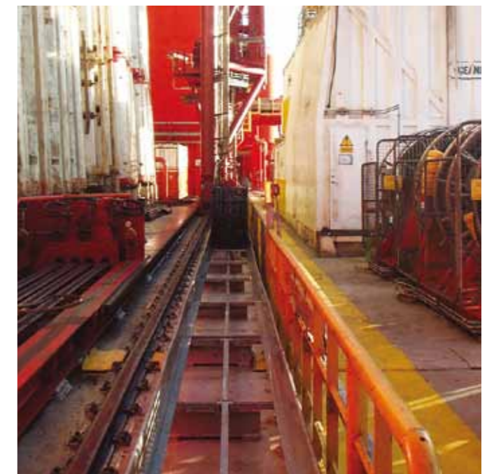
E4 Series 600 extension link – long travel application onboard West Navigator (Norway)
