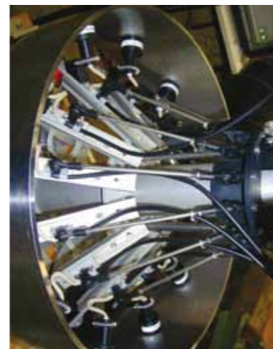
Linear guides and tie bars
