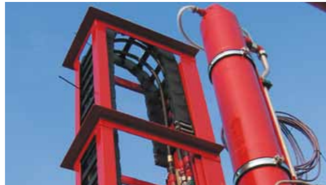
Vertical boom on a riser handling crane for AKMH (West E Drill)
