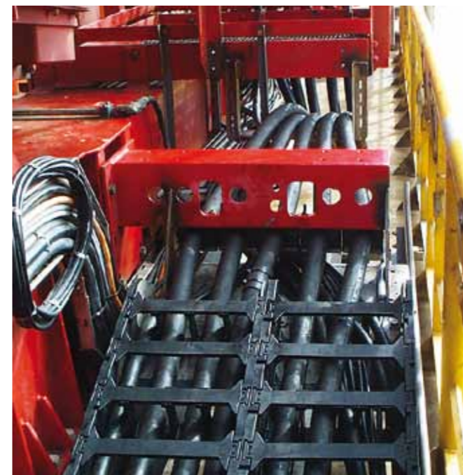
Light weight AND high stability: Polymer e.chain® tames stiff hydraulic hoses.
