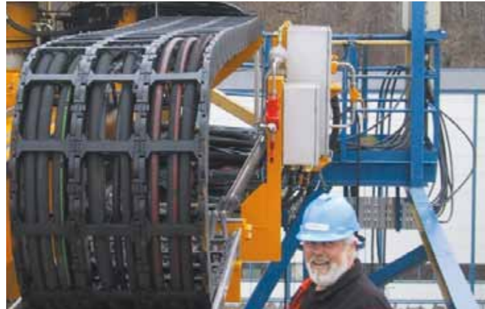
Strong, modular, corrosion resistant and easy to install: igus® e.chains® for heavy fill weights in harsh offshore environment
