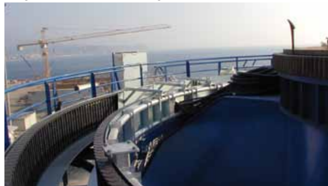
Low maintenance and long service life: igus® e.chain® series 5050 with reverse bend radius on port crane equipment
