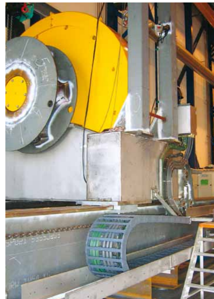
ATEX version igus® e.chainsystem®, series E4, harnessed with hydraulic hoses and igus® chainflex® cables. Here shown on a test stand, now in operation on Dalia FPSO (linear motion of mooring)
