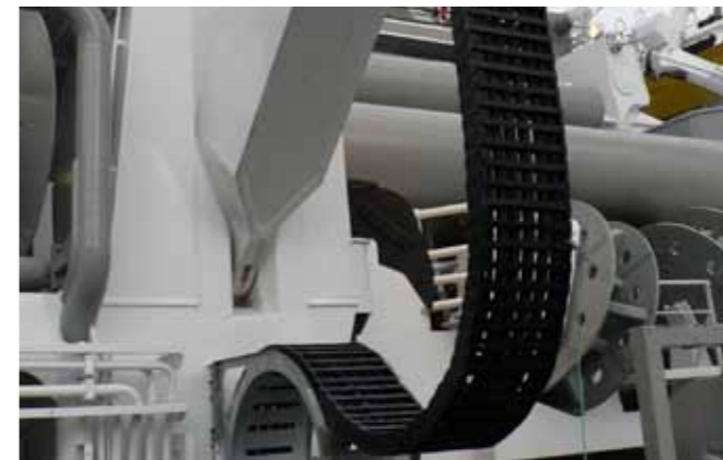
e.chain® with reverse bend radius guides cable and hose package on A-frame onboard anchor handler
