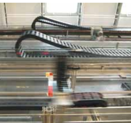
Push Pull forces speed up to 10 m/s, acceleration up to 200 m/s² are tested
